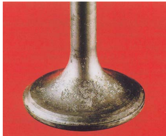
Figure 2 - Fuel Sulphur Damage
